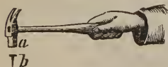
A MAGNETIC HAMMER. a represents the hammer attracting to it the tack b.
